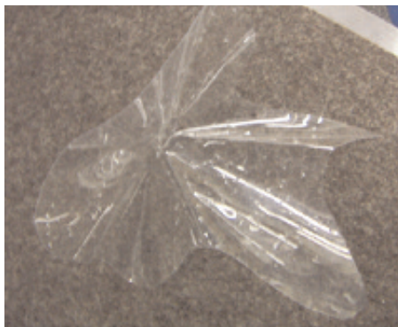
Unpainted piece formed with .007" Dura-Lar
