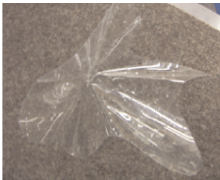
Unpainted piece formed with .007" Dura-Lar
